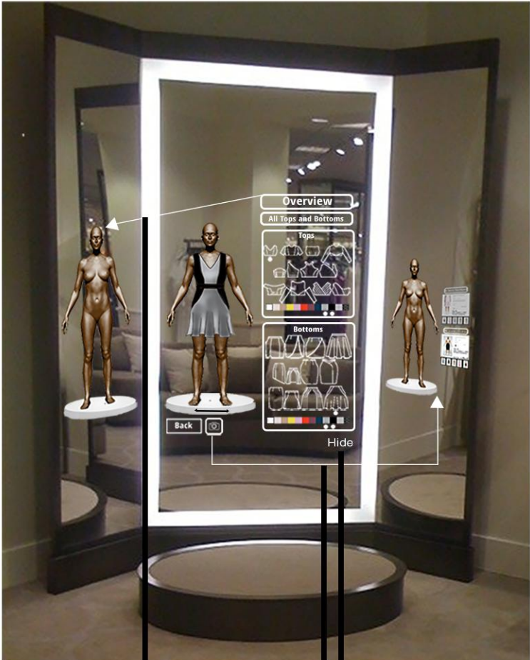
The smart mirror allows multiple screens to be shown by dragging them to parallel mirrors.
